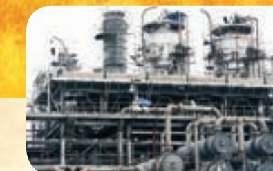
High pour-point lube-stock coolers. Designed for minimum size and high wall temperature to overcome pour-point effects. Design & fabrication: Heat Exchangers International, Australia. Contractor: LG Industries Courtesy: Thai Petrochemicals
