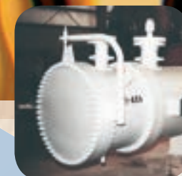
HCGO/tempered water cooler. High wall temperature achieved to limit pour-point effects. 1 shell only needed. Courtesy: Imperial Oil, Canada
