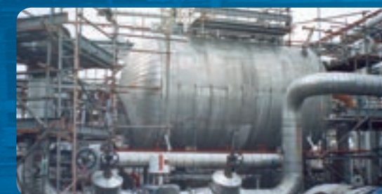
Ethylene vapouriser, Malaysia. Courtesy: Optimal Chemicals
