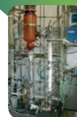
Thermosiphon reboiler studies. University of Braunschweig
