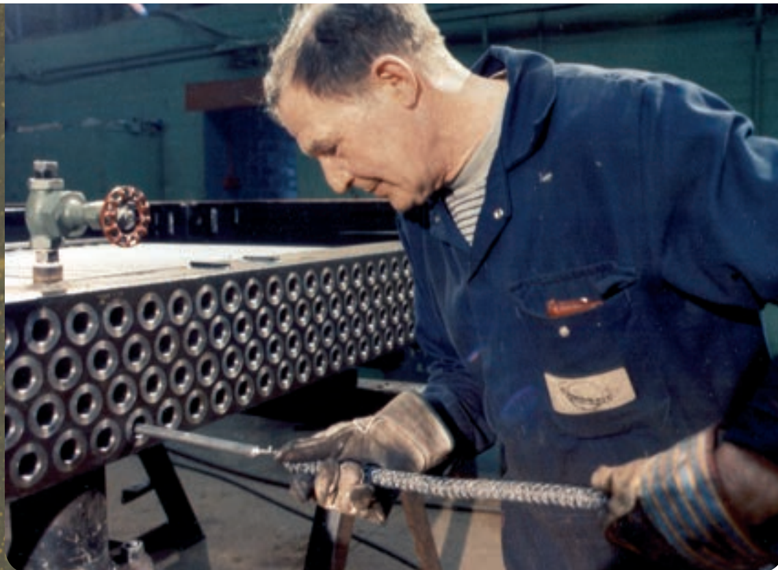
Air-cooler for Shell Oil, Nigeria, fitted with hiTRAN Matrix Elements in less than 3 hours.
